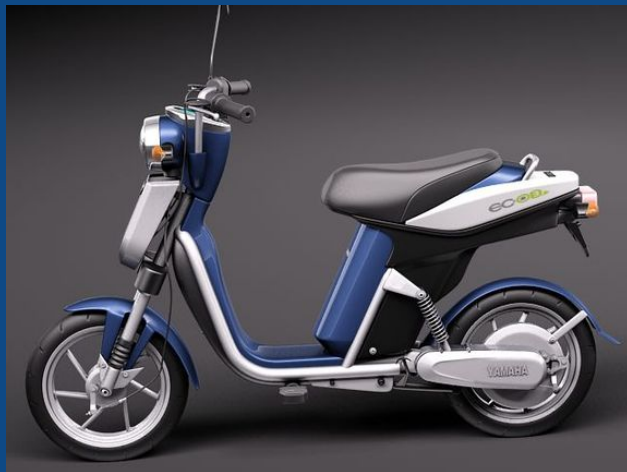
Yamaha electric moped 56 kg 1.4kW 40+ km range
