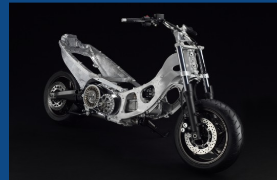
Yamaha Tmax Aluminium frame Central engine
