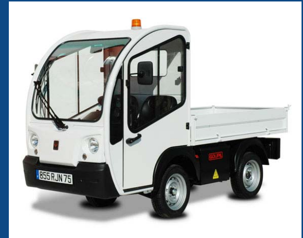
Goupil G32 Engine 12 kW, 100 km range
