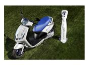
• **E-Vivacity**, 100% electric new generation 60 kms autonomy / 45 km/h / lithium-ion battery / 2 boots
