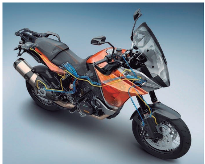
KTM has fitted its newest model with Motorcycle Stability Control, a new ABS system that allows emergency braking in curves and provides additional stability to the vehicle.
