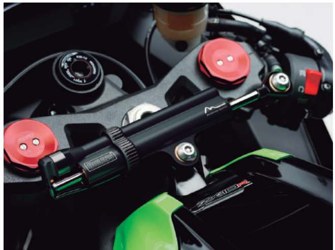
Kawasaki's Ninja ZX-10R is as standard equipped with an Electronic Steering Damper, substantially improving steering control.
