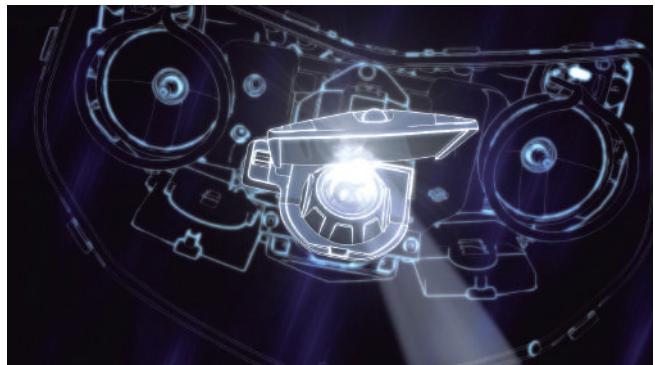
BMW Motorrad adaptive headlights improve road visibility when cornering at night, significantly increasing active safety.
