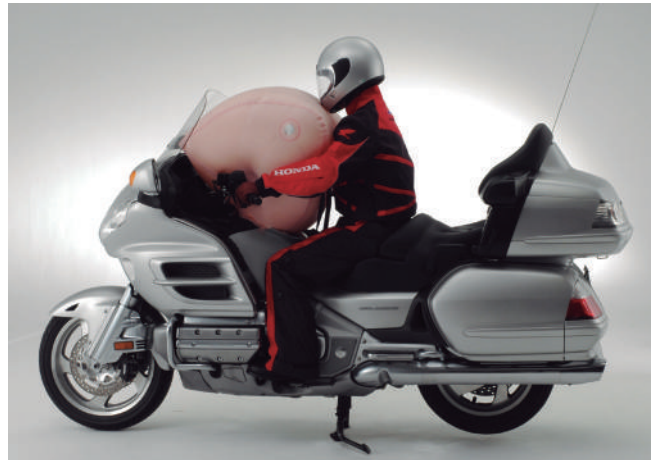
In 2006, Honda launched the world's first production motorcycle air-bag system on the Honda Goldwing. The system helps to lessen the severity of injuries caused by frontal collisions.
