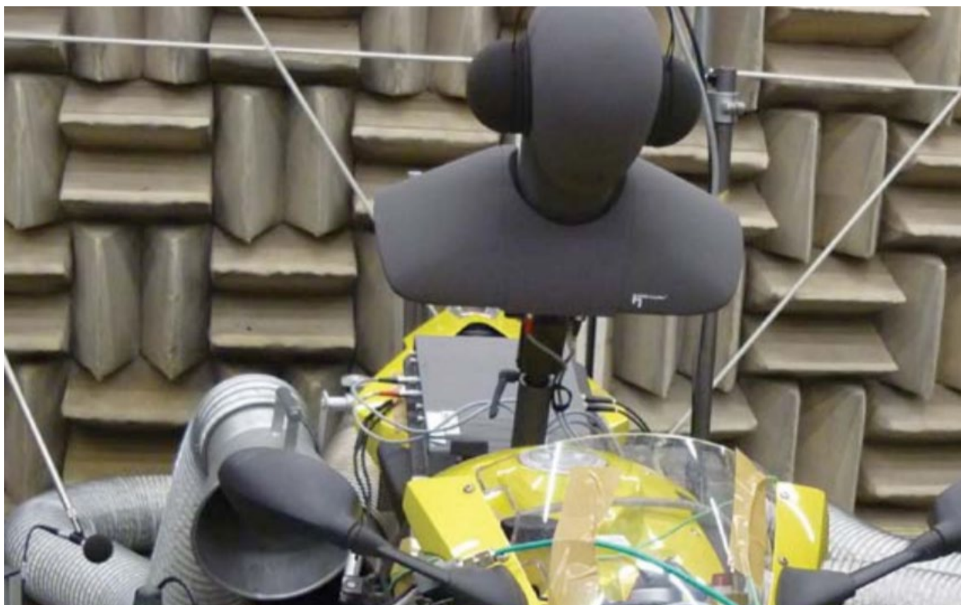
The testing of PTW sound is governed by UNECE Regulation 41, that sets the overall sound limits and includes the Additional Sound Emission Provisions (ASEP).
